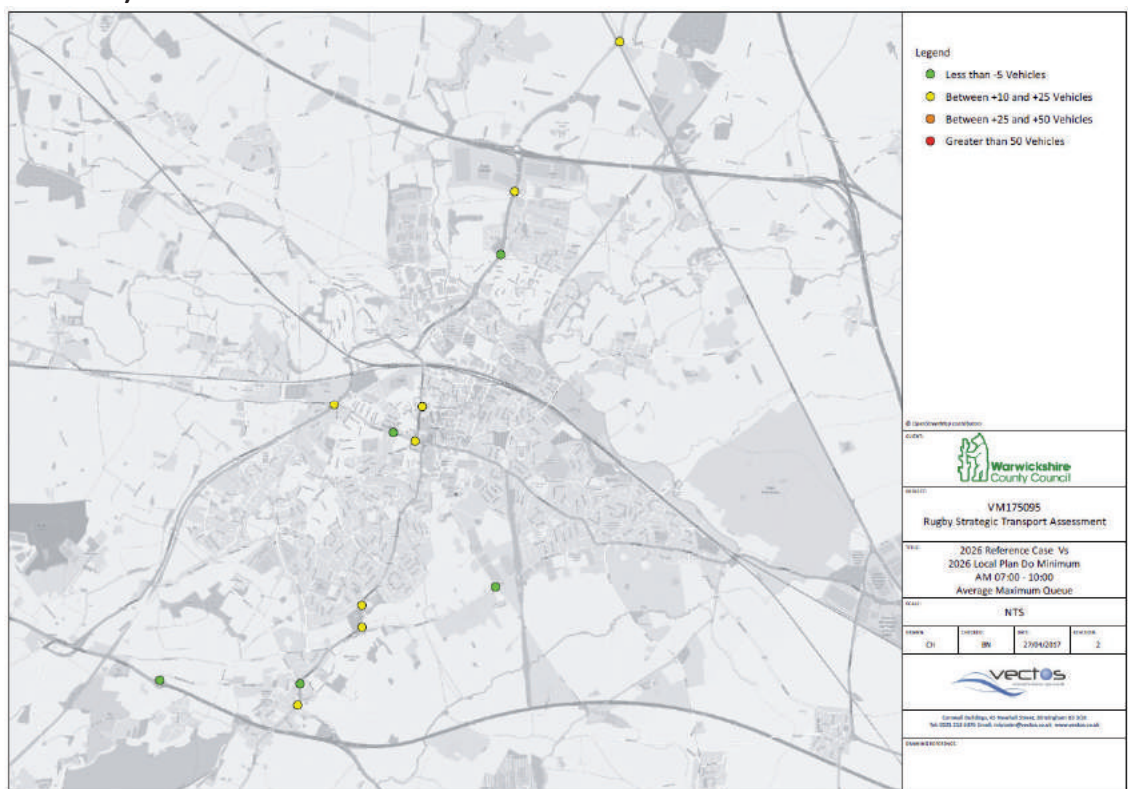
Figure 35 AM Period Maximum Queue Length Comparisons (Ref vs. Local Plan Do Minimum)
