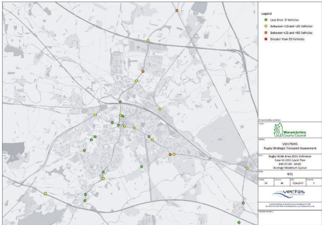
Figure 20 AM Period Maximum Queue Length Comparisons (Ref vs. Local Plan)
