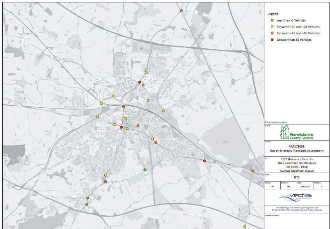
Figure 36 PM Period Maximum Queue Length Comparisons (Ref vs. Local Plan Do Minimum)
