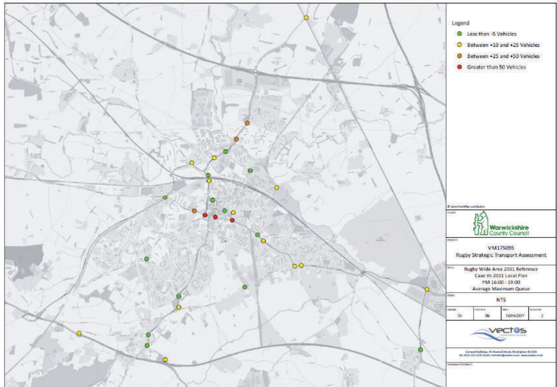
Figure 21 PM Period Maximum Queue Length Comparisons (Ref vs. Local Plan)
