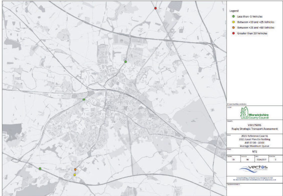
Figure 24 AM Period Maximum Queue Length Comparisons (Ref vs. Local Plan Do Nothing)
